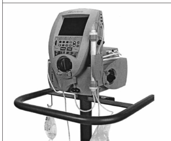
Figure 2: An ultrafiltration console
